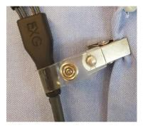
Place the ground electrode on e.g. the wrists.
