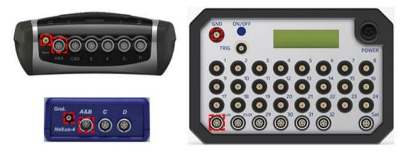
Sensors can be disconnected by pulling the silver ribbed part of the connector backward.
