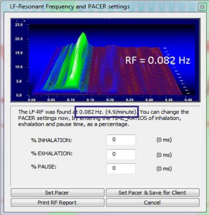
Set the PACER setting by entering the time ratios (1), based on the found RF, and press 'Set Pacer' (2).
