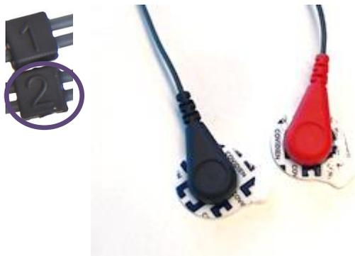
Snap an electrode on to the EXG ground snap-on.
