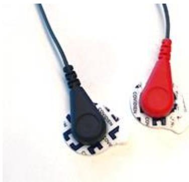
Place the red (positive) and black (negative) electrodes on to the skin at the position of interest. Make sure the electrodes at the muscle of interest are placed parallel to the muscle fibers. The orientation of the positive and negative snap-on is not critical, they can be mutually swapped. Usually the electrodes are placed right next to each other.
