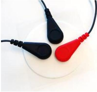
When using un-gelled electrodes apply conductive gel on to the EMG triode triode electrode
