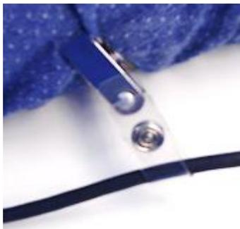
Place an EMG TP electrode on to the EXG ground TP.
