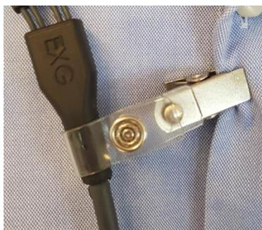
Snap the EMG electrode on to the EXG ground snap-on.
