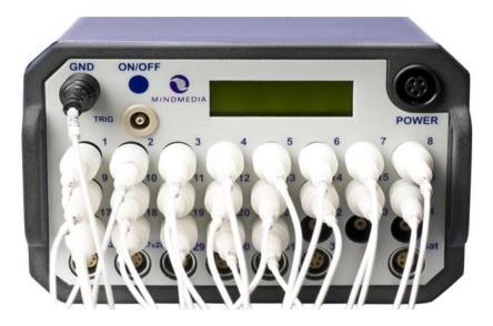
Snap the NeXus EEG cap in to NeXus EEG Cap Adapter. The connectors will only fit one way.
