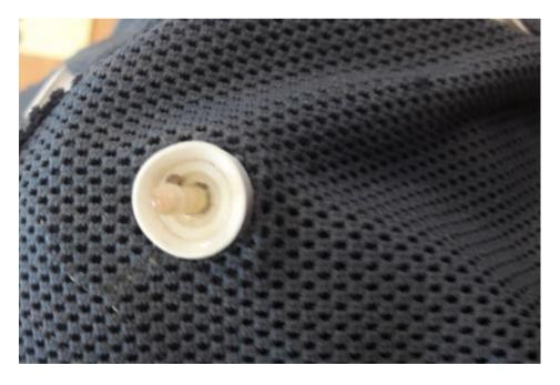
When drying the cap, make sure the connector of the cap doesn't hang beneath the wet cap to prevent the connector getting wet. To speed up drying a hair blower can be used. Make sure not to hold the hair blower to close to the cap.
