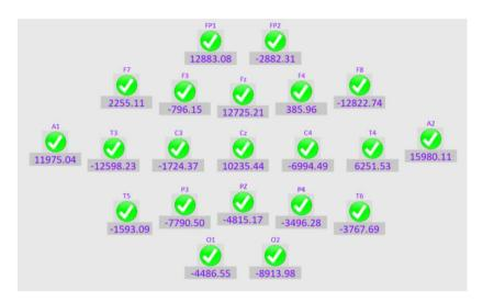
The electrode contact values supply an indication of signal quality.
