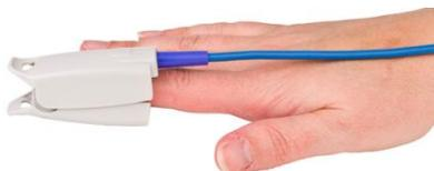
When using the Blood Volume Pulse Head sensor with an (ear)clip, it can also be attached to a finger. Please note that signal quality is poorer than with the Blood Volume Pulse Sensor.
