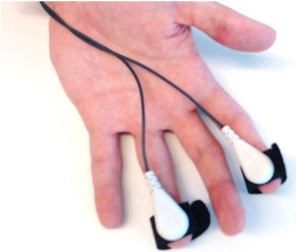
Alternatively place the Skin Conductance electrodes on the middle phalanges (middle of the fingers) of the non-dominant hand, at the palmar side of the fingers.
