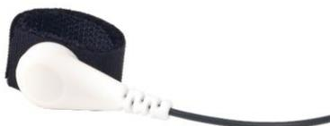
Usually the Skin Conductance electrodes are placed on the fingertips of the non-dominant hand, at the palmar side of the fingers. Try to standardize which fingers are used.
