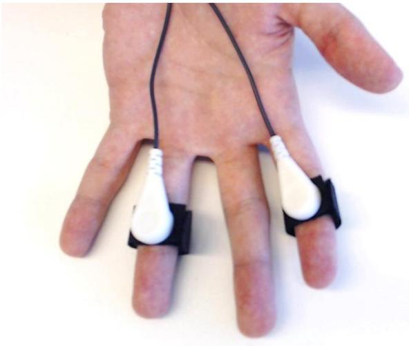
Optionally secure the cables to the hand with some tape to avoid movement artifacts.
