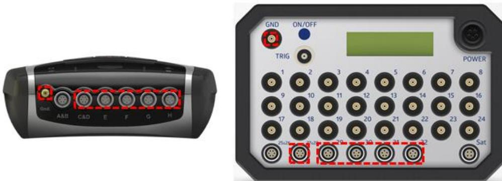
Connect the EXG Ground to the Ground (Gnd) of the NeXus.
