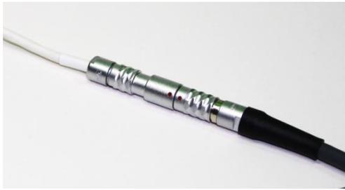
Place Minicap electrodes on to the red EXG sensors TP and place a Minicap electrode on to the EXG ground TP. Slightly twist the connector in to EXG TP connection in order to make good connection.
