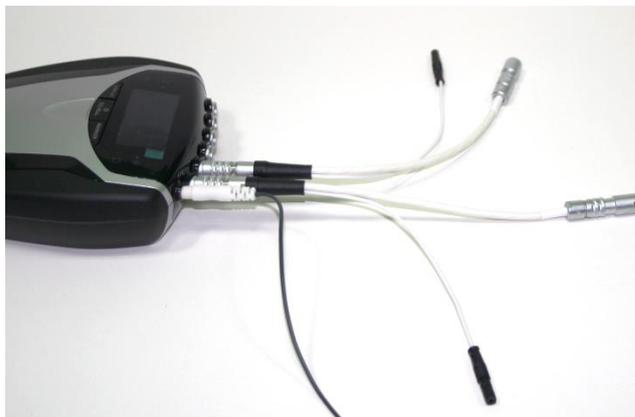
Connect the black connectors of the two Linked ear cables by using the small black tube.
