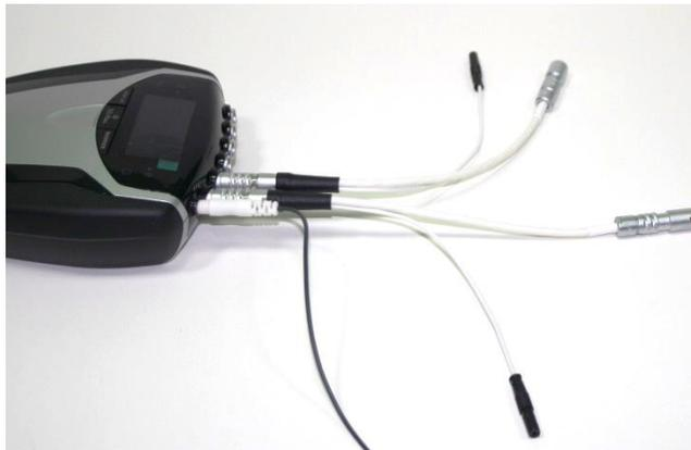
Connect the black connectors of the two Linked ear cables by using the small black tube.
