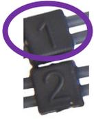
Place the black snap-on of pair one of the EXG sensor and the ground snap-on together with disc electrodes on to an ear clip.
