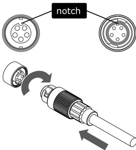
Connect the power supply cable into the power supply socket on the front of the device (POWER).
