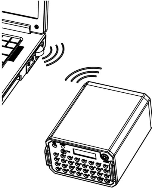
1. Insert the Bluetooth dongle in a USB port. Wait for Windows Update to install the drivers for the Bluetooth dongle.
