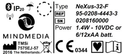
The device label can be found at the bottom of the device (example of device label is shown here). It contains the REF code, Serial Number, power requirements and other properties of the device. Use the REF number to look up the channel specifications as listed in [chapter 8](#).
