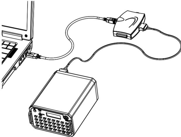
1. Connect the optical fiber to the input of the Fusbi and the other end to the fiber connector on the NeXus-32. It does not make a difference which connector goes where.
