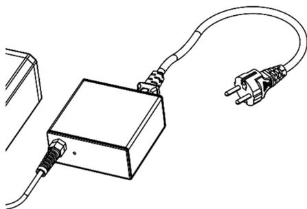
Check that the power supply is labeled as 'SUP3'. Connect the mains cable to the power supply and the other side into a well-grounded power outlet. The LED on the power supply will light up green.
